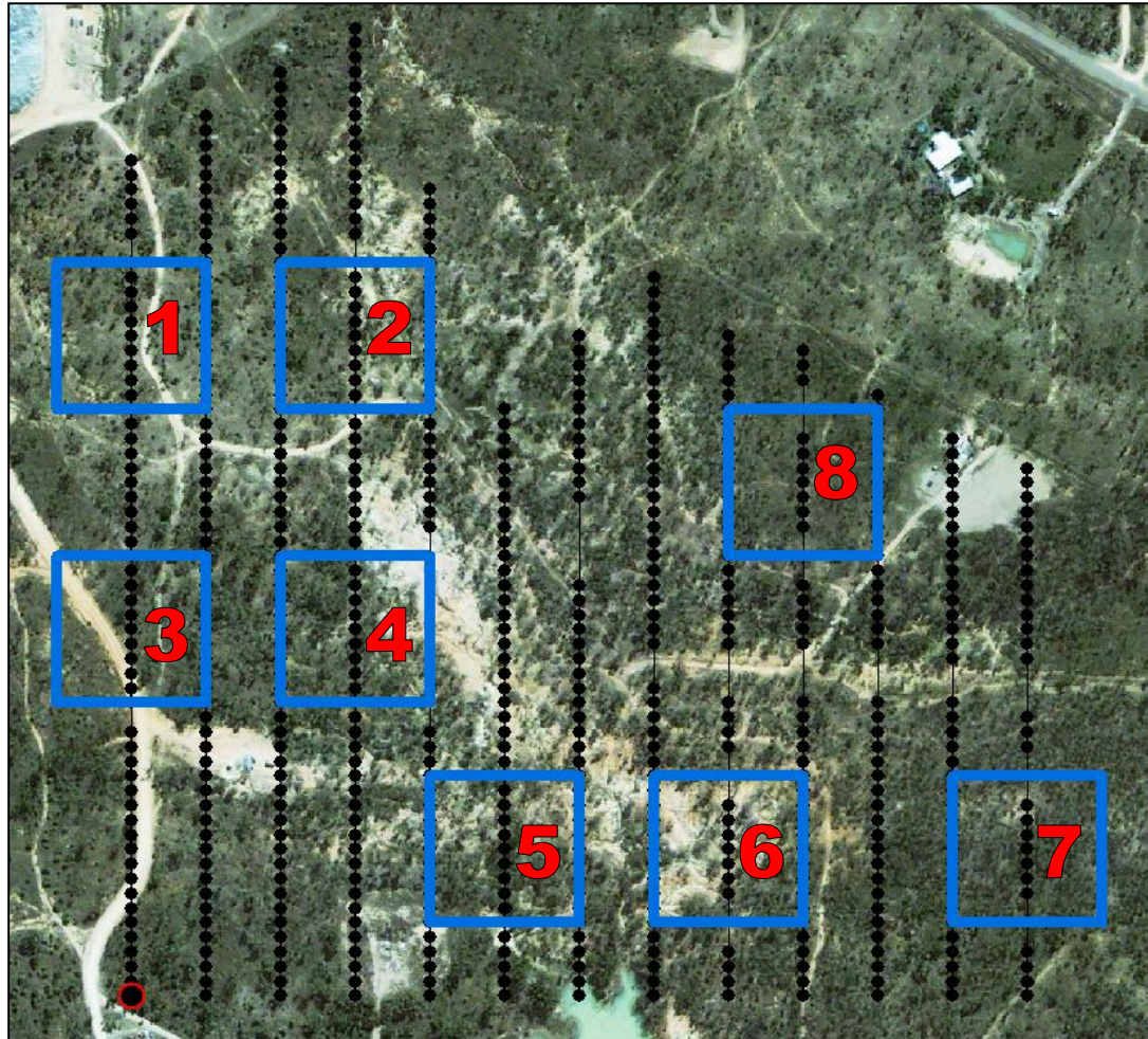
Fig. 3: Location of 2011 small loop surveys. Two to four lines were surveyed with each of the eight loops. For further details on the July/Aug survey plan, see Section II. Loops are outlined in bold blue and numbered in red while the receiver stations are black dots.
